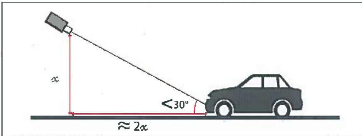
For optimal functioning, the camera should have at least a slight vertical angle to avoid direct illumination from the sun.
